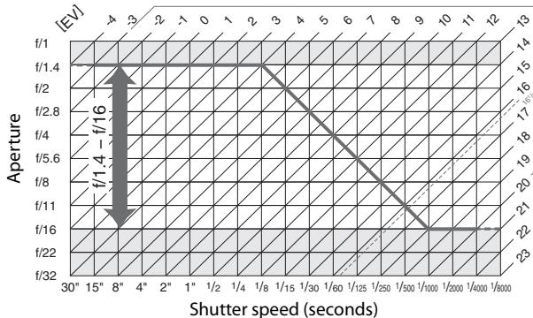
The maximum and minimum values for EV vary with ISO sensitivity; the above graph assumes an ISO sensitivity of ISO 100 equivalent. When matrix metering is used, values over  $16 \frac{1}{3}$  EV are reduced to  $16 \frac{1}{3}$  EV.
